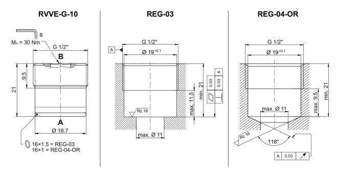
RVVE-G-10 = check valve / screw-in cartridge valve
