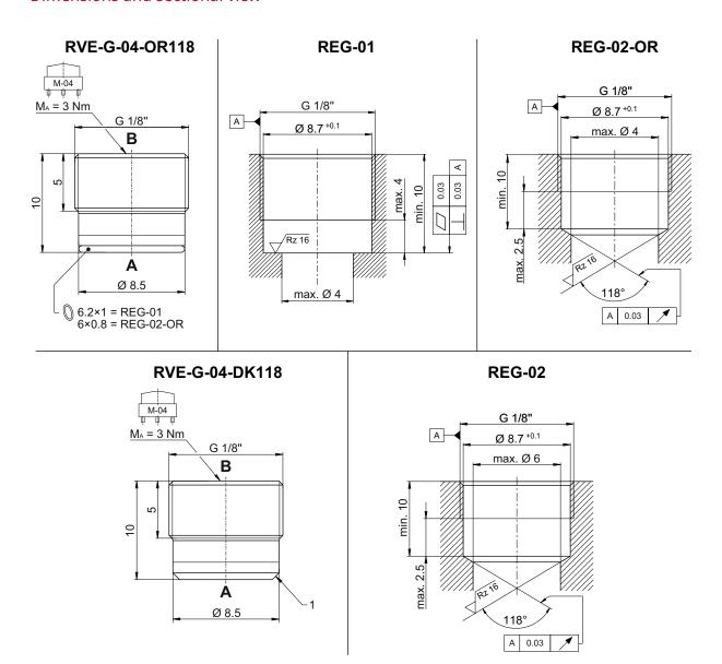
**RVE-G-04** = check valve / screw-in cartridge valve
